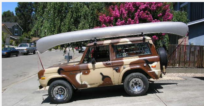
Canoe Antenna —Timothy Sammons, N6CC, San Ramon, CA 17 foot aluminum canoe mounted on black plastic rack-mounts = a quarter wave horizontal mobile antenna for the 20 meter Ham band. It worked fine with a little help from impedance matching!
