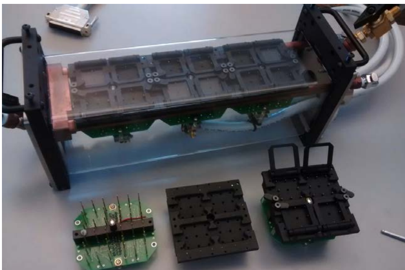
Above: One test unit of the SPA system can enable the simultaneous study of 12 1"x1" devices.
