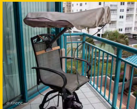
"My Super Stealth Bar Stool Tower and Fire Pit Cover for the MFJ-1786. From a distance [the loop antenna] looked like a patio chair with an umbrella..." Robert Goodman K3RRR
